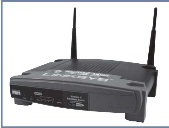
A Linksys WiFi (802.11g) wireless router. Such a router allows WiFi enabled laptops and desktops to connect remotely to it within a given range.
