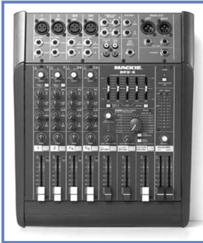
A Mackie 4 channel mixer unit. Note the four white channel faders at the bottom left of the mixer.
