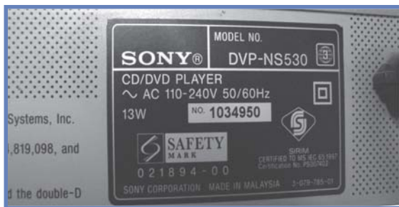
The serial number of the equipment is usually mentioned on a label on the side, back or underside of the equipment. Note that the label also gives information regarding power ratings.
