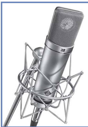
A Neumann U 87 condenser studio microphone. Note the suspension shock mount that holds the microphone and prevents accidental movements of the mic from causing a rumble in the audio.
