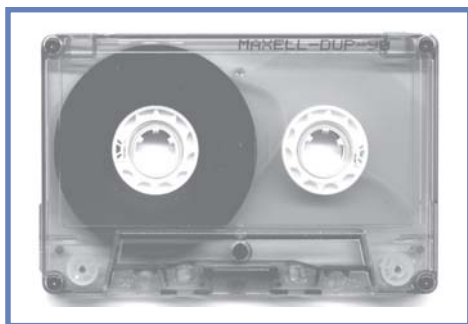
A typical audio cassette, also known as a compact cassette. The tape ribbon is contained in a transparent plastic shell.
